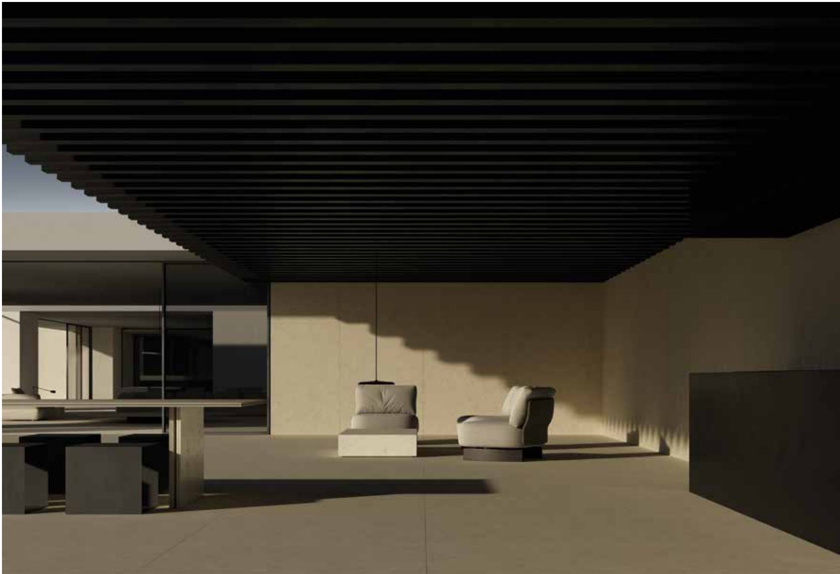
Img. Facade: Luna Light Grey Soft Crafted 120x270x6mm (48"x106") Exterior flooring: Luna Light Grey BHAS 120x120x9mm (48"x48") Lithotech Countertop: Luna Light Grey Soft Textured
