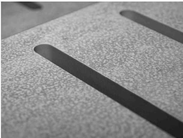
Image. Detail of the water-jet process on a swimming pool grating.
